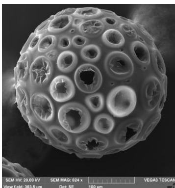
Image 1. SEM image of the GMA resin obtained using toluene dispersion of Fe 3 O 4 nanoparticles.
